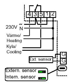
**NB:** The thermostat may control either heating or cooling, but not both simultaneously.
